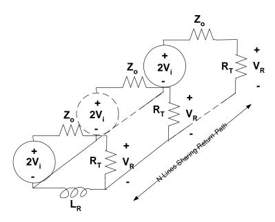
The incident voltage,  $V_i$ , however is not  $V_S$  but it is the noisy  $V_S$ , i.e.  $V_S$  with the transmitter signal return cross-talk taken into account:  $V_i = V_S(1 - K_{XRT})$ . Again, we solve this circuit by superposition. (Note: our termination at the receiver is matched to the line,  $R_T = Z_o$ .)
