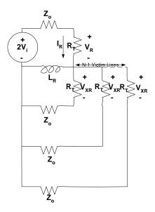
We can now solve for  $V_{XR(total)}$  by first solving for  $V_R$ . We find  $V_R$  by simple voltage division:
