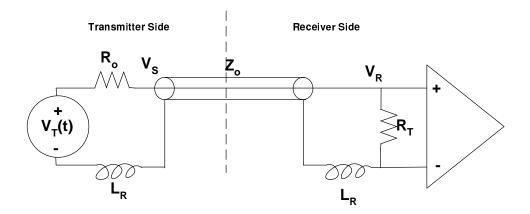
We have N lines sharing the return path. We want to solve for the signal return cross-talk,  $k_{xr}$ . As hinted in the problem, we can treat the transmitter and receiver side separately, as denoted in the figure above.
