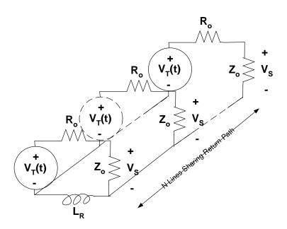
We solve for the transmitter signal return cross-talk,  $K_{XRT}$  exactly as done in the problem session: Solving by superposition for the voltage,  $V_X$  induced across each of the other N-1 lines, we have the following circuit:
