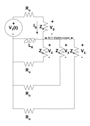
$\mathbf{Z}_{X}$ , the equivalent impedance for the parallel network, i.e.  $\mathbf{L}_{R}$  in parallel with the other N-1 lines, is:
