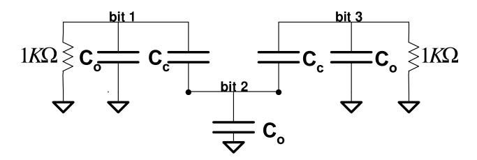
Since the voltages on lines 1 & 3 will be exactly the same, we draw an equivalent circuit as:
