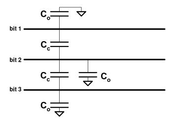
Note: We are ignoring the coupling capacitance to other neighboring and non-adjacent bit-lines. Initially all of the bitlines are precharged to a value of 1 V. We then pull bits 1 and 3 down with the pull-down circuit shown, which we model as a 1  $k\Omega$  resistor. Constructing an equivalent circuit, we have:
