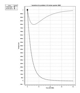
A comparison between the actual voltage waveform on bit-line 2 and our estimated waveform on bit-line 2 shows that the estimation used in the first option gave us a close approximation to the actual behavior.
