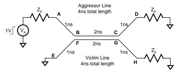
Using this information, sketch and dimension the voltage waveform at the far-end of the victim line (point H). You may ignore any effects that lead to waves with less than 10mV amplitude.
