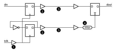
In this one, we no longer are sampling our data twice, both in phase and 90 degrees from that, in order to compensate for skew. Instead, we assume that both lines have very little skew, such that we can clock to data exactly in the center of the eye. In this sense, we now see the skew of the transmission line, and the transmit flip flops and drivers. The only thing we will have cancelled would be the jitter of the transmit clock buffer tree.
