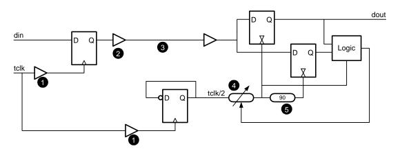
In this one, this is similar except for a few things. First, the jitter of the transmit clock buffer tree is included, since both paths have different amounts of jitter.(Since they have different clock buffers) Everything else will be exactly similar to part(A), as the skew from (2) and (3) will be compensated by the per pin closed loop timing.
