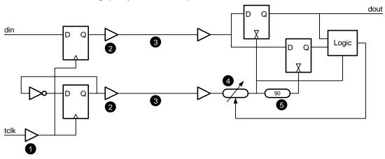
The figure above illustrates a 1Gb/s closed loop timing system with five sources of delay, skew, and jitter identified by white numbers in black circles. The sources are:
